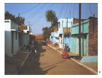
Roads Have positively downward slopes from high poinrts to drainage courses and are thus able to act as storm water channels and attenuate the rain peaks.
