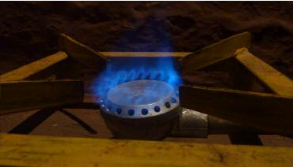
Gas from the biogas system used for cooking purposes
